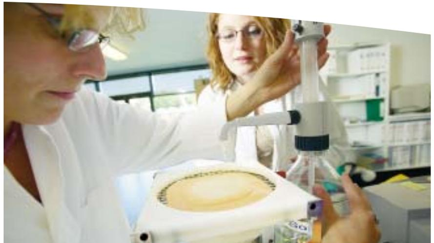
Project manager Mette Irene Kolte (right) and laboratory assistant Rikke Marie Torpe with the equipment used to measure absorption capacity.
